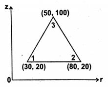
9. The nodal coordinates for an axisymmetric triangular element shown in fig are given below. Calculate the strain-displacement matrix for that element
