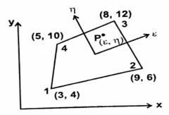
4. For the four noded quadrilateral element shown in fig determine the Jacobian and evaluate its value at the point  $(1/2, \frac{1}{2})$
