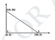
7. Calculate the element strains for an axisymmetric triangular element shown in fig the nodal displacement are.  $u_1 = 0.001$ ,  $u_2 = 0.002$ ,  $u_3 = -0.003$ ,  $w_1 = 0.002$ ,  $w_2 = 0.001$  and  $w_3 = 0.004$  all dimensions are in mm.
