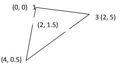
5. Find the temperature at point (1, 1.5) inside a triangular element shown with nodal temperature given as  $T_i = 40^{\circ}$ C,  $T_j = 34^{\circ}$ C and  $T_k = 46^{\circ}$ C. Also Calculate the location of the 42°C contour line for triangular element shown in fig.
