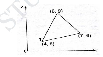
8. For an axisymmetric triangular elements as shown in fig. Evaluate the stiffness matrix. Take modulus of elasticity E = 210 GPa. Poisson's ratio = 0.25. the coordinates are given in millimetres.
