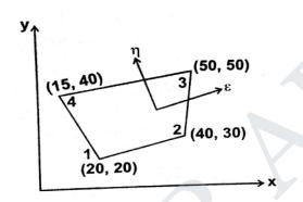
5. Evaluate the Jacobian matrix at the local coordinates  $\varepsilon = \eta = 0.5$  for the linear quadrilateral element with its global coordinates as shown in fig. Also evaluate the strain-displacement matrix.
