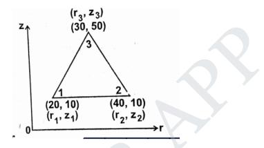
10. A long hollow cylinder of inside diameter 100mm and outside diameter 120mm is firmly fitted in a hole of another rigid cylinder over its full length as shown in fig. The cylinder is then subjected to an internal pressure of 2 MPa. By using two element on the 10mm length shown calculate the displacements at the inner radius tame E = 210 GPa.  $\mu = 0.3$  (BT3)
